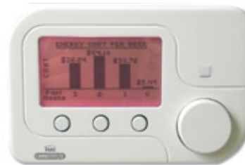
This graph allows you to monitor your Energy Cost, broken down by a specified time determined by your energy company.*
